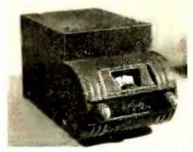
RCA model 8M for instrument panel mounting has 5 tubes—lists for \$19.95.
