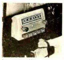
Safety tuning with mechanical push buttons selecting five stations is featured by Crosley for less than \$25.
